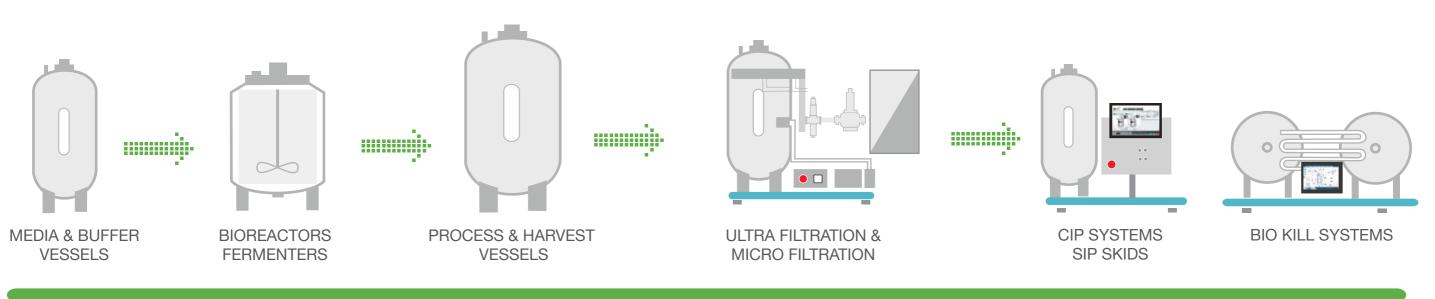
We design equipment to match your process requirements. As an end to end solution provider we start by mapping your process followed by designs which meet your exacting requirements. Our product portfolio includes media and buffer preparation vessels, bioreactors and fermenters, filtration system, harvest and process vessels, media and sterile filtration skids. Our solutions include CIP, SIP and bio-kill systems.
